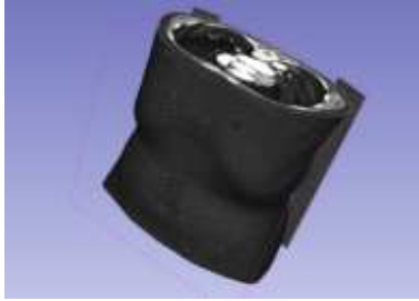
Figure 10: The regional cut: Defining a region of interest enacting a straight cut. Slicer v4.10.2 (screenshot)
